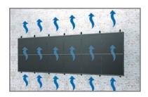
Cooling effect of module rear ventilation provides stable power and yields.
